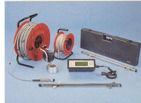
Inclinometer probe and readout
